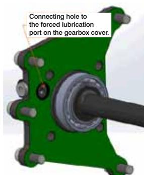
Furthermore, the flange offers also the option to bring pressurized oil to the PTO through an external pipe. In fact, outside on the flange there is a plug G 1/4, which can be removed for the connection of an external pipe.
